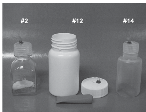
FIGURE 1. Three different drug chamber and desiccant bag combinations utilized in the study. The symbols of the combinations are the same as used in Table 1: #2 polycarbonate/latex, #12 HDPE/silicone, #14 polypropene/PVC. The humidity sensors has been glued into the caps of the chambers.
